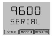
The secondary display will show BAUD and will then scroll SERIAL PORT BAUD RATE after 10 seconds.
