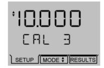
The correct values should be entered and saved as for the 1 point calibration. When all chosen buffer types have been entered and confirmed the instrument display will update to show the next set up menu option.
