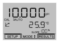
If a successful I point calibration has been performed the secondary display will momentarily show CAL OK. The slope value from the calibration will be displayed. The instrument will then update the display.
