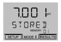
The instrument will store: Primary pH or mV readings
