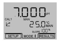
If a successful I point calibration has been performed the secondary display will momentarily show CAL OK. The instrument will then update the display. The display will then show the next part of the calibration sequence if a 2 and/or 3 point calibration has been selected. If a 1 point calibration only is required the instrument will return to the main measuring screen. Eo is shown on the status display
