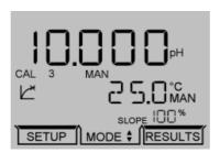
If a successful I point calibration has been performed the secondary display will momentarily show CAL OK. The instrument will then update the display.
