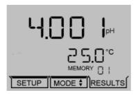
The Up arrow increments the memory index, the Down arrow decrements the memory index.
