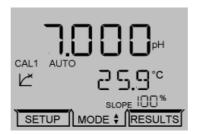
If a successful I point calibration has been performed the secondary display will momentarily show CAL OK. The instrument will then update the display. The display will then show the next part of the calibration sequence if a 2 and 3 point calibration has been selected. If a 1 point calibration only is required the instrument will display the Eo value on the status screen and then return to the main measuring screen.
