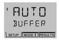
The secondary display will show BUFFER and will then scroll BUFFER TYPE after 10 seconds. Select the type of buffer from the options available by scrolling through the list using the Up/Down arrows – AUTO, MAN, JIS, NIST or DIN. (AUTO relates to the Jenway buffer types supplied with the instrument).
