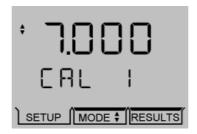
with the first digit of the value flashing. Adjustment of the flashing digit can be made using the Up/ Down arrow keys. The Left/Right arrow keys are used to select the next adjusting digit which will flash when selected. Once the full reading has been adjusted to the correct value, press the STO key. If a 1 point calibration only is being performed the instrument display will update and show the pH Resolution set up menu.
